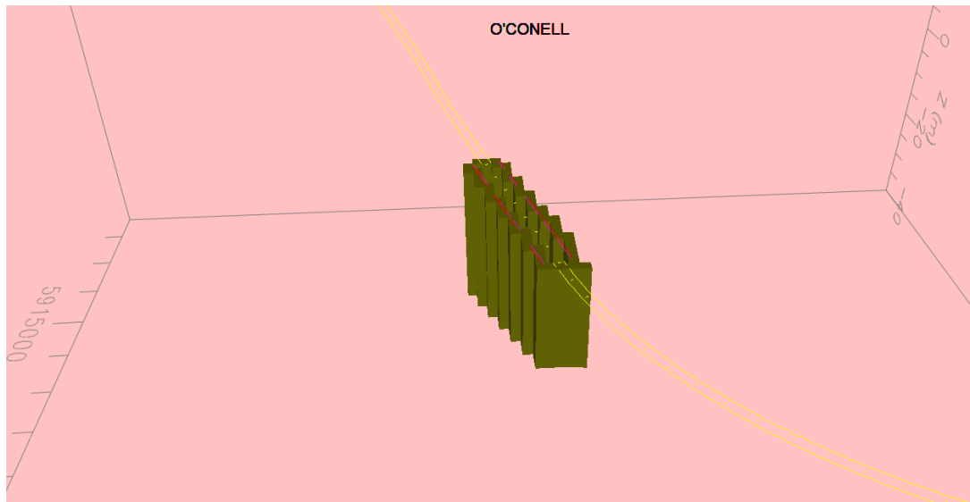
Figure 5-34. 3D view of the diaphragm walls. O'Connell
